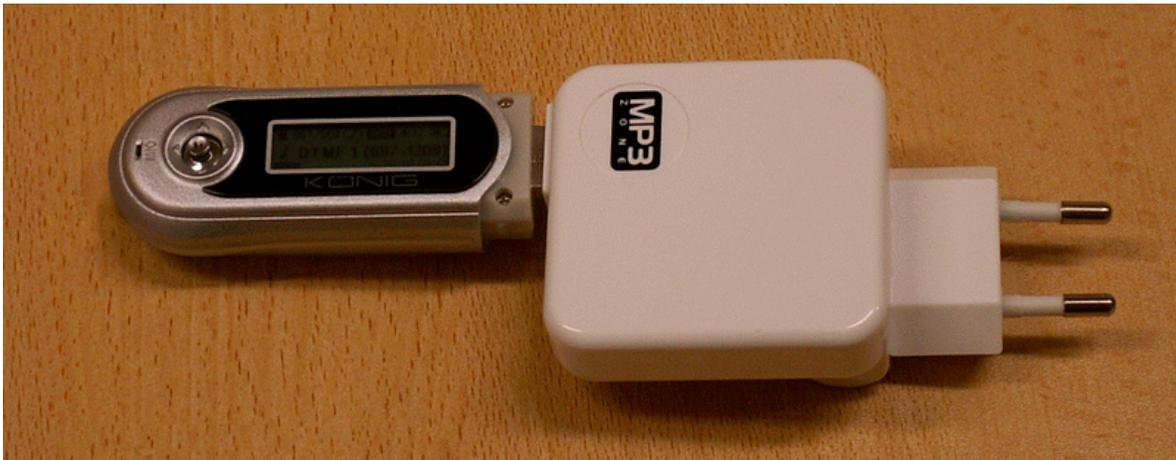
**Figure 2. MP3 player with an embedded FM transmitter, connected to power adapter. (The antenna is not attached.)**
